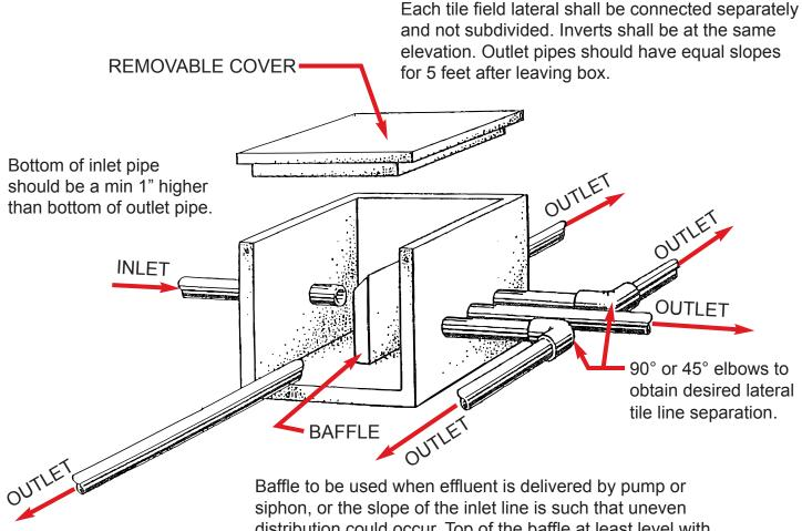
distribution could occur. Top of the baffle at least level with the crown of the inlet pipe.
